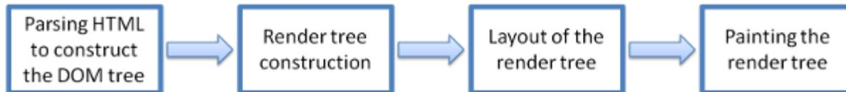
**Figure 2:Rendering engine basic flow.**
