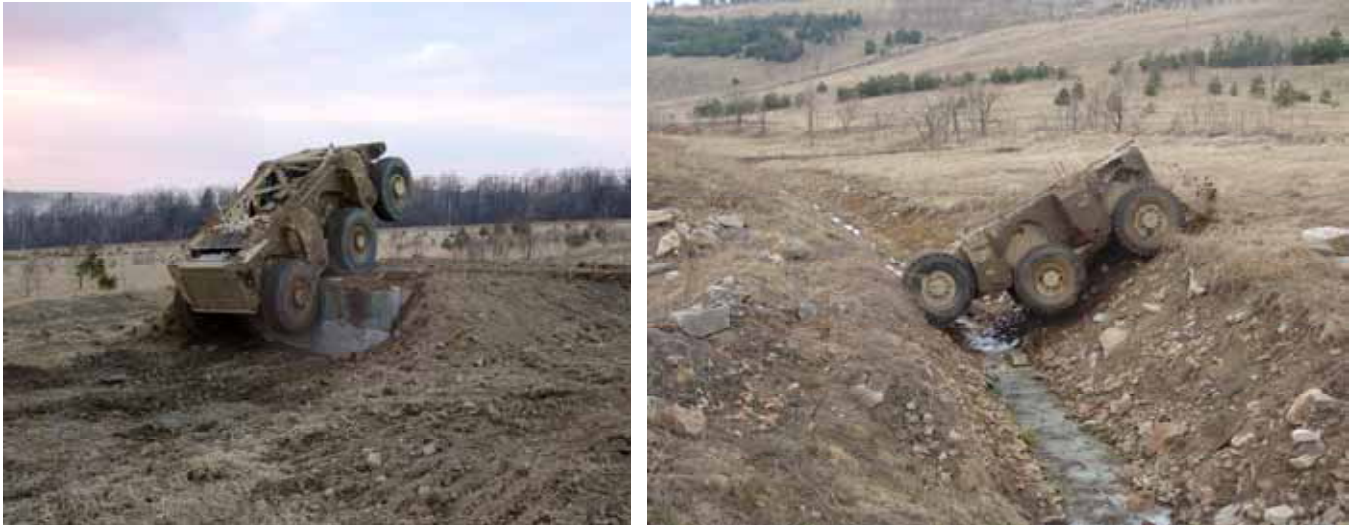
Figure 2: Crusher breaching an obstacle (left) and crossing a ditch (right).
