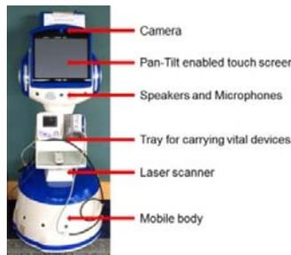
**Fig. 3.** The kiosk type robot platform, Charlie. It consists of a camera, a Pan-Tilt enabled touch screen, speakers, microphones, ultrasonic sensors, bumper sensors, a laser scanner, two single board computers and a 24V Li-Polymer battery.
