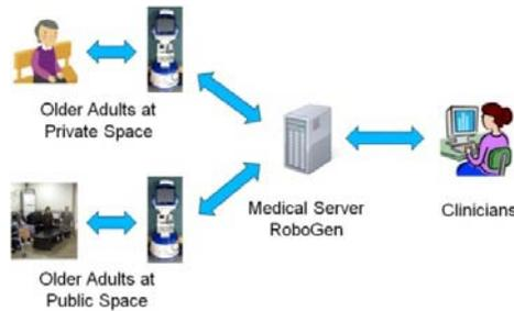
**Fig. 2.** Overview of the healthcare robot system, Healthbots. Robots help older adults in various spaces and send information such as vital signs and interaction records to the medical server, RoboGen. Doctors and psychologists access the medical server and check the health status of the older adults.
