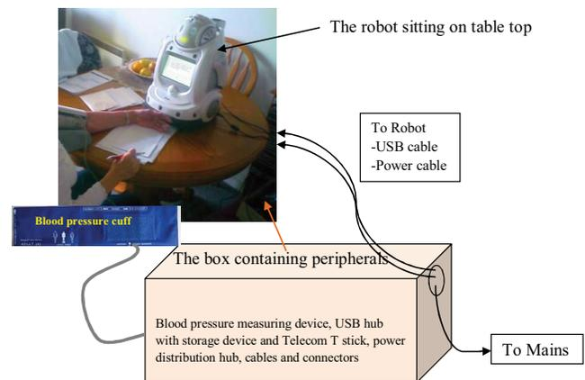
Fig. 2. Setup of the robot at older participants' independent living
